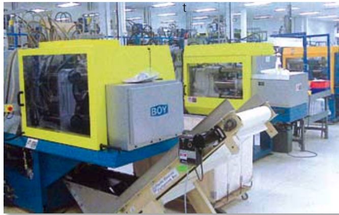
25 BOY injection molding machines are still working at the LSR molding department of Limtech
