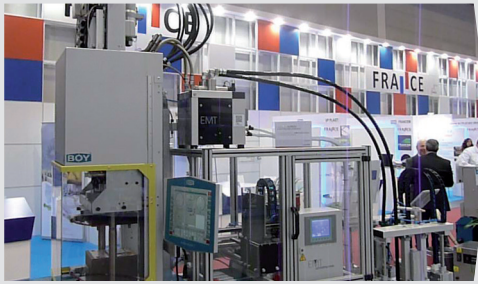
Automated LSR overmoulding. Integrated removal handling
