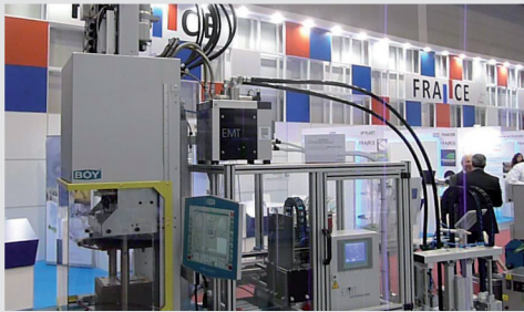
Automated LSR overmoulding. Integrated removal handling
