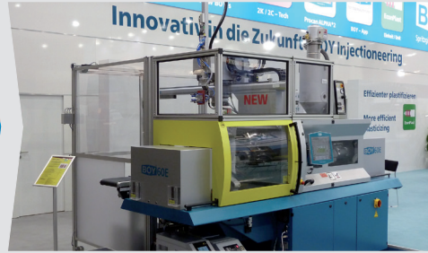
Production cell with CE-compliant safety housing
