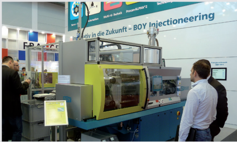
Production cell with CE-compliant safety housing
